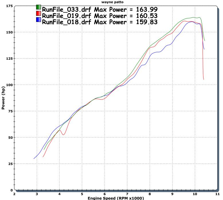
■ RunFile\_018.drf - 04/03/2011 11:24:46 Run Type: RO Run Conditions: 36.02 °C, 29.77 in-Hg, Humidity: 33%, STD: 1.04 4th gear test std tyre 15/41 Max Power = 159.83
