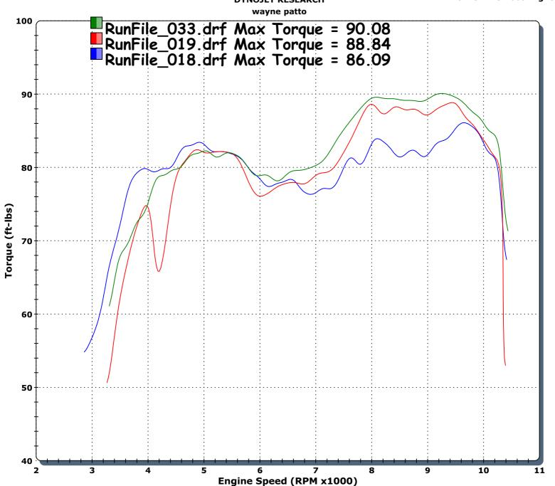
RunFile\_018.drf - 04/03/2011 11:24:46 Run Type: RO Run Conditions: 36.02 ℃, 29.77 in-Hg, Humidity: 33%, STD: 1.04 4th gear test std tyre 15/41 Max Torque = 86.09 2009 Ducati Streetfighter, "Std Headers, race filter with race scoops, Tboy termi style ecu, Carbon slip-ons. Powercommander and both cyl's Dyno-Tuned.
