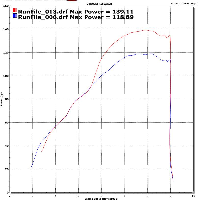
RunFile\_006.drf - 29/07/2009 2:53:06 PM Run Type: RO Run Conditions: 69.28 F, 30.65 in-Hg, Humidit y: 43%, STD: 0.98 Max Power = 118.89
