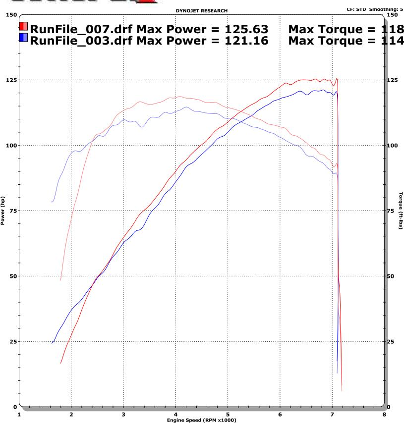
RunFile\_003.drf - 11/03/2008 5:10:48 PM Run Type: RO Run Conditions: 87.01 F, 30.01 in-Hg, Humidit y: 52%, STD: 1.03 Max Power = 121.16 Max Torque = 114.63 M109R Boulovard.Cobra long Staggerds.
