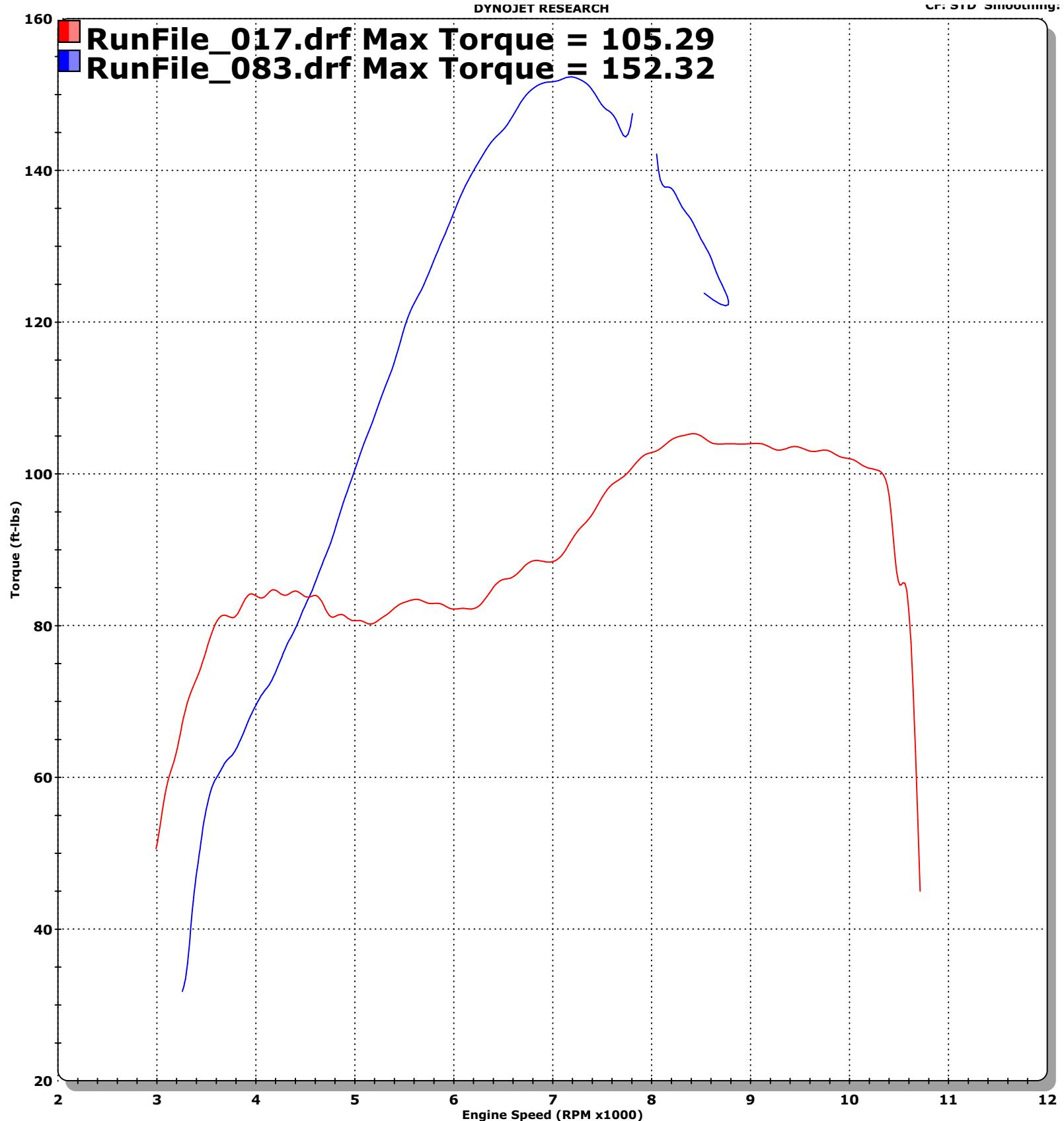
RunFile\_083.drf - 19/10/2007 9:12:16 AM Run Type: RO Run Conditions: 73.81 °F, 30.39 in-Hg, Humidity: 41%, STD: 0.99
