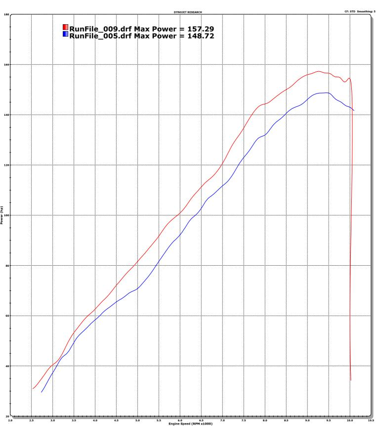
RunFile\_005.drf - 20/04/2011 6:13:52 PM Run Type: RO Run Conditions: 24.00 ℃, 30.38 in-Hg, Humidit y: 54%, STD: 1.00 Max Power = 148.72
