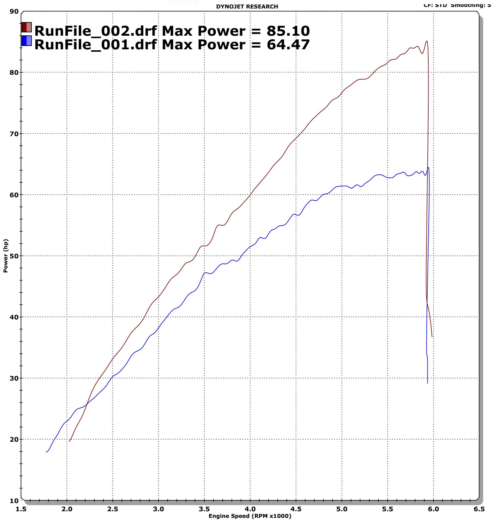
RunFile\_001.drf - 19/11/2008 4:14:22 PM Run Type: RO Run Conditions: 82.65 °F, 29.86 in-Hg, Humidity: 40%, STD: 1.02
