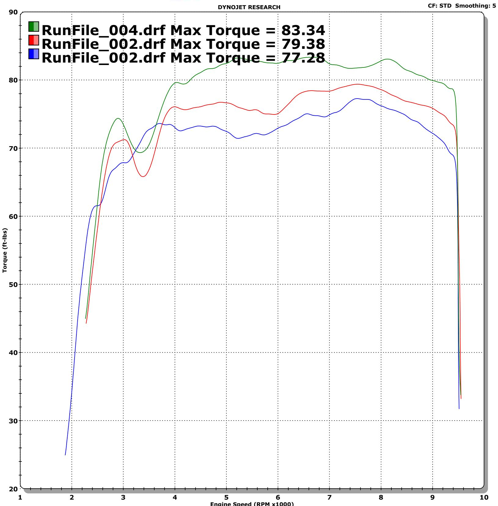
■ RunFile\_002.drf - 4/04/2007 2:40:42 PM Run Type: RO Run Conditions: 86.02 °F, 30.08 in-Hg, Humidity: 36%, STD: 1.02
